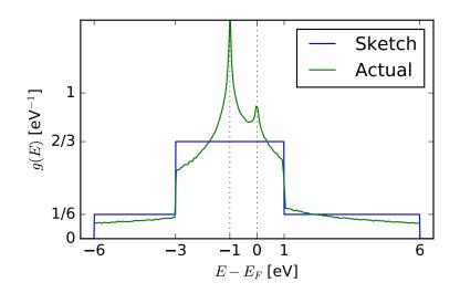
For reference, I have also shown the actual density of states from the model I used to construct the band structure for comparison. Note the spikes at 0 and -1 eV: these correspond to the flat sections in the center of each band at the X point of the band structure. We could have also guessed this part, but we got quite close with just the simple considerations above.
